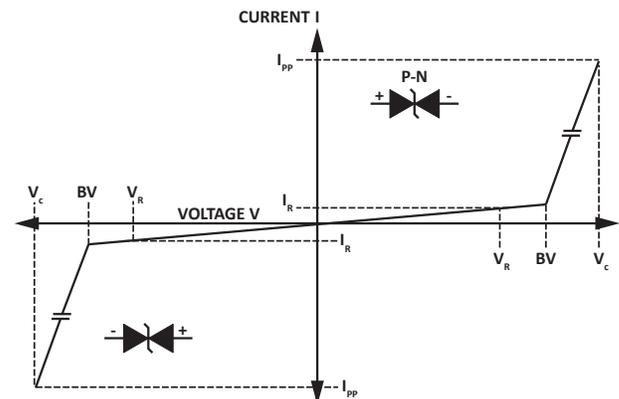
Figure 4. Bidirectional V-I Curve
