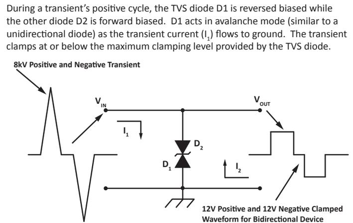
Figure 3. Bidirectional Device (Symmetrical Clamping)
