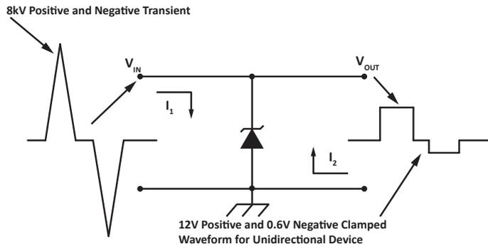
Figure 1. Unidirectional Device (Asymmetrical Clamping)
