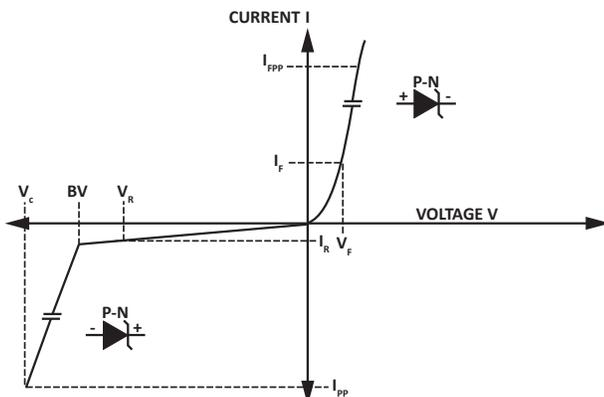
Figure 2. Unidirectional V-I Curve
