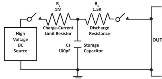
Figure 1. Test Circuit for HBM ESD, MIL-STD-883, Method 3015
