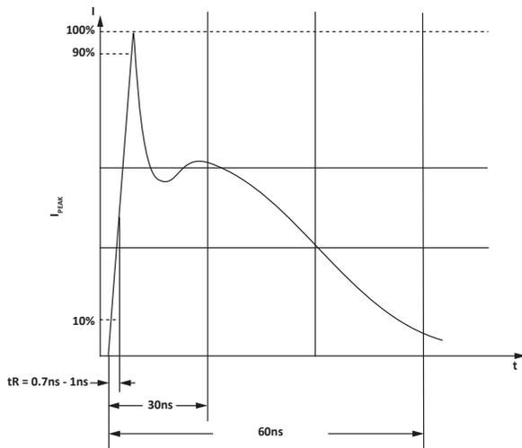
Figure 4. Current Waveform for HBM ESD for IEC 61000-4-2
