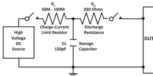
Figure 3. Test Circuit for HBM ESD for IEC 61000-4-2
