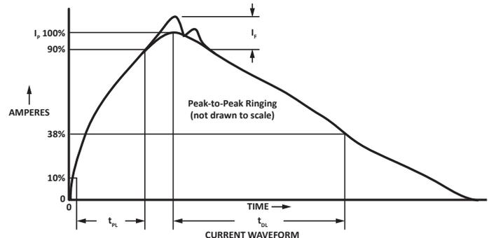
Figure 2. Human Body Model Current Waveform for MIL-STD-883, Method 3015
