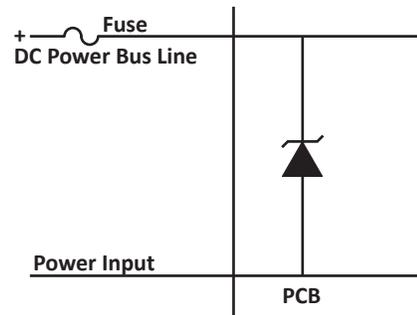
Figure 3. Fuse Location Relative to the TVS Device
