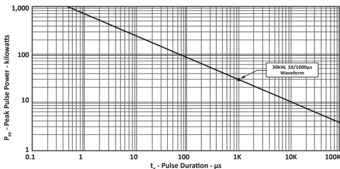
Figure 2. Peak Pulse Power vs Pulse Time
