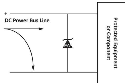
Figure 1. Current Path for Shorted Surge Suppressor
