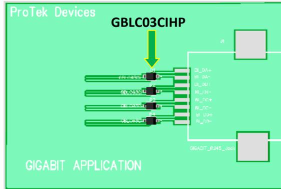
**Figure 2 - Gigabit Protection Using the GBLC03CIHP**
