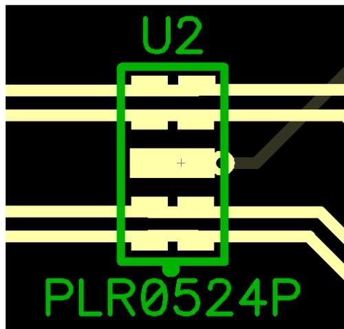
**Figure 5 - Enlarged View of the PLR0524P**
