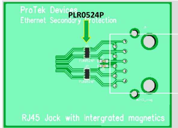
**Figure 4 - Integrated Connector Using the PLR0524P**
