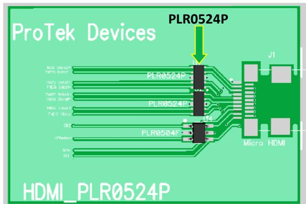
**Figure 2 – TMDS Data Line and Clock Protection Using the PLR0524P**
