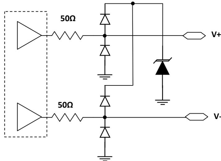
**Figure 1 - TMDS Pair Protected by Using the PLR0524P**
