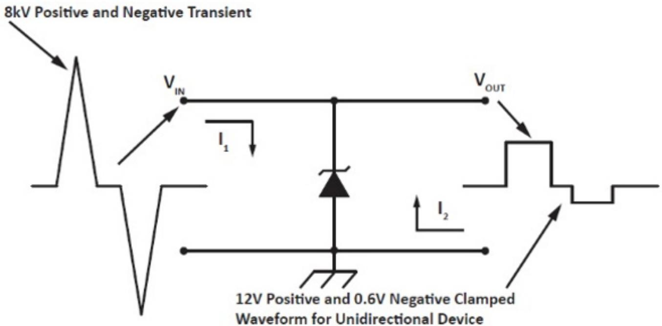
Figure 2 shows an electrical transient current being diverted to ground. Under normal operating conditions, the TVS diode presents a high impedance path to the protected circuit. During the transient event, the TVS diode achieves breakdown. It then presents a low impedance path, which shunts the transient current through the TVS diode device.
