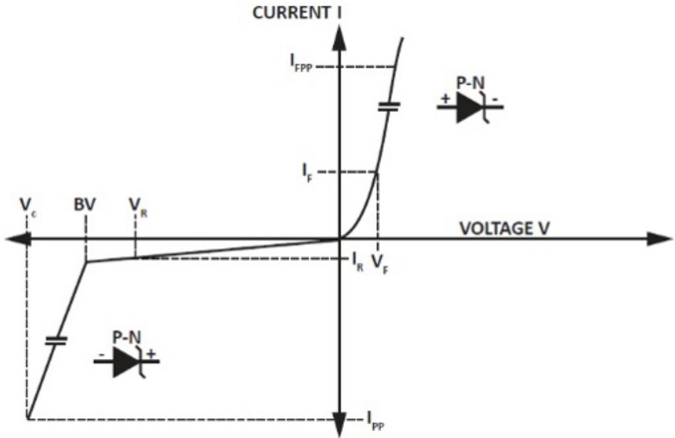
The V-I curve shown in figure 1 is similar to that of a Zener diode. However, TVS diodes are designed and characterized for transient voltage suppression, while Zener diodes are designed and specified for voltage regulation. With a TVS diode, an electrical transient is clamped instantaneously and diverts the damaging current away from the protected device.
