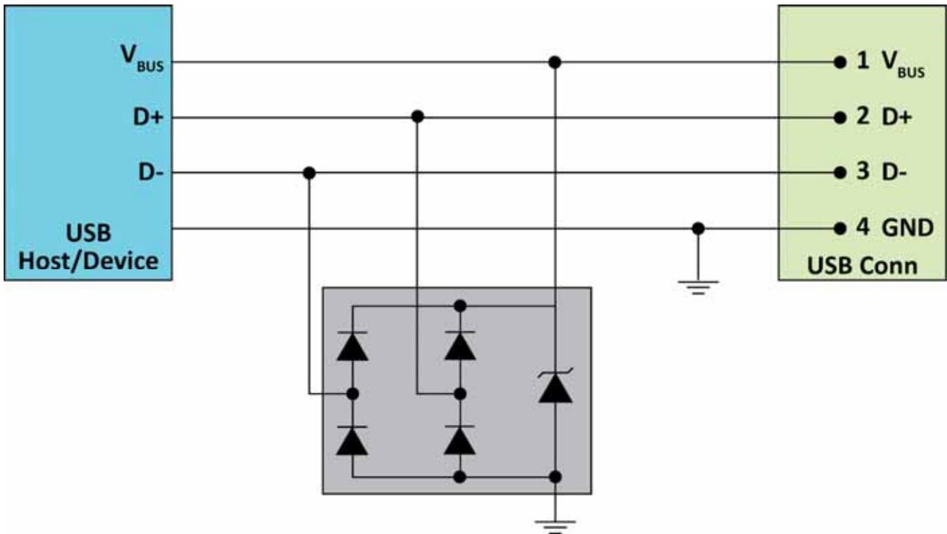
*Example USB 2.0 Interface Circuit Protection Diagram Using a Combo Steering Diode / TVS Array*
