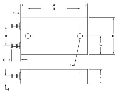
$\textbf{Note:} \ \textbf{Recommended torque value for mounting:} \ \textbf{less than 10 inch pounds}$
