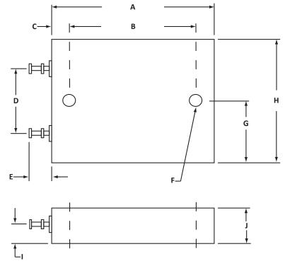
Note: Recommended torque value for mounting: less than 10 inch pounds
